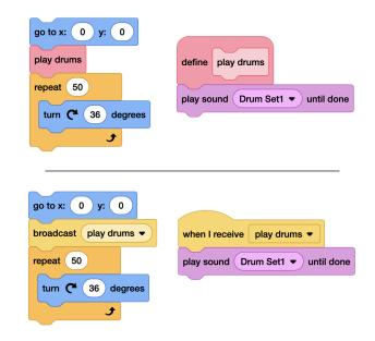
Try these two code sequence pairings to see the difference between calling for a custom block and calling for a broadcast.
